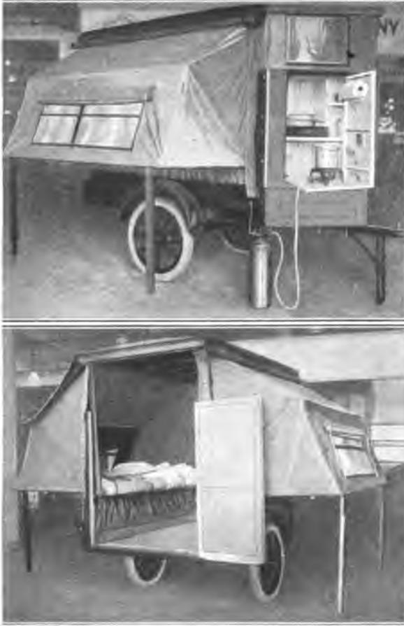
Two Views of a Well-Designed Touring Trailer: The Canvas Extensions Fold Inward, and the Telescoping Sides Permit the Top to be Lowered
