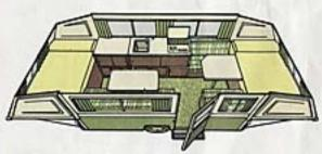
Romada Specifications: Weight, 1740 lbs.\* • Length, 16'61/2" • Width, 6'71/6" • Road Height, 53" • Tires, 20.5x8.0—10", 6-ply-rated. Living Area: Height, 6'2" • Width, 6'51/2" • Length, 20'7" • Bed Dimensions, 72" x 54".
