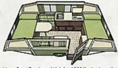
Mesa Specifications: Weight, 1390 lbs.\* • Length, 13'1/2" • Width, 6'77/8" • Road Height, 53" • Tires, 20.5x8.0-10", 4-ply-rated. Living Area: Height, 6'2" • Width, 6'51/2" • Length, 16'1" • Bed Dimensions, 72" × 48".
