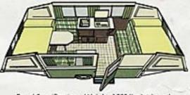
Royal Specifications: Weight, 1590 lbs." • Length, 14'101/4" • Width, 6'77/8" • Road Height, 53" • Tires, 20.5x8.0—10", 6-ply-rated, Living Area: Height, 6'2" • Width, 6'51/2" • Length, 19' • Bed Dimensions, 72" x 54".
